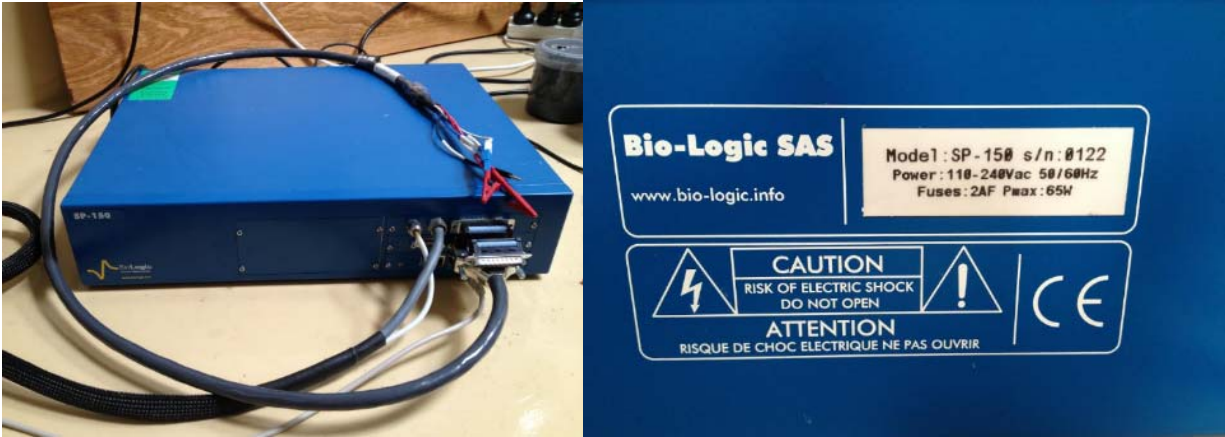
Figure 4. The Bio-Logic SP-150 potentiostat for LPR testing
